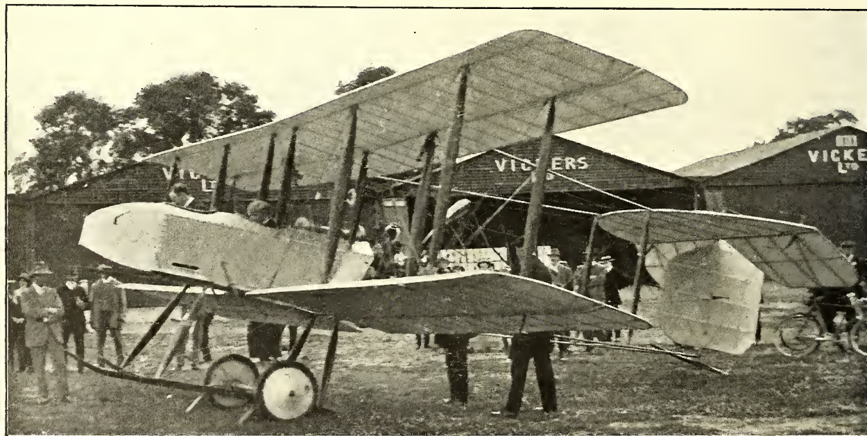
The latest Vickers gun-carrier (100-h.p monosoupape Gnome) about to start at Brooklands, piloted by Mr. Harold Barnwell.
